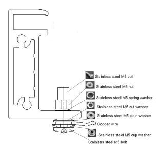
Fig. 12 Grounding the aluminum frame with copper wire
