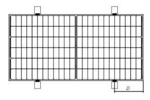
Fig. 4 Rails vertical to the long-side frame
