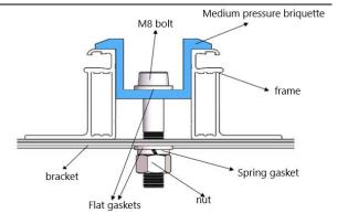
Fig. 10 Installation schematic diagram of mid clamp
