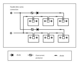
Fig. 11 Schematic diagram of electrical connection
