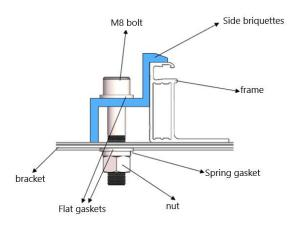
Fig. 9 Installation schematic diagram of fringe clamp
