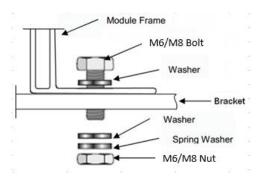
Fig. 2 Diagram of the bolt installation process
