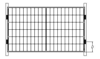
Fig. 5 Rails overlapping the short-side frame
